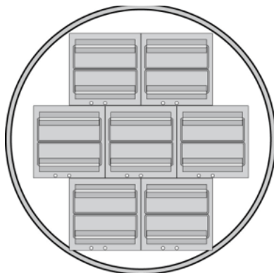
S-1500AB stainless steel, standard square rack configuration. 9,100 vial capacity
